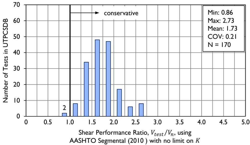
**Figure 2-35: Shear Performance Ratio calculated using the AASHTO Segmental Procedure (2010) with no limit on  $K$  for beam tests in the UTPCSDB-2011 Evaluation Database-Level II (from Nakamura (2011)).**
