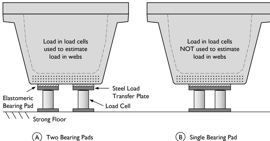
**Figure 6-12: Bearing conditions used in U-Beam load tests.**
