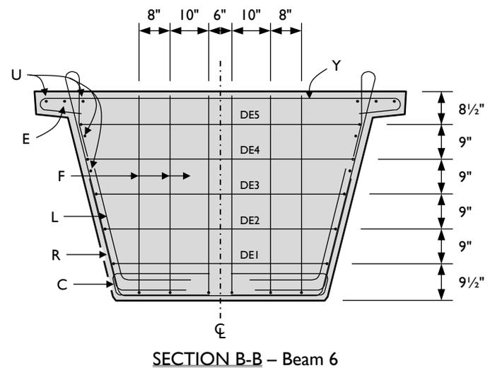
Figure A-32: Beam 6 end-region plan views and cross-sections (1 of 2).
