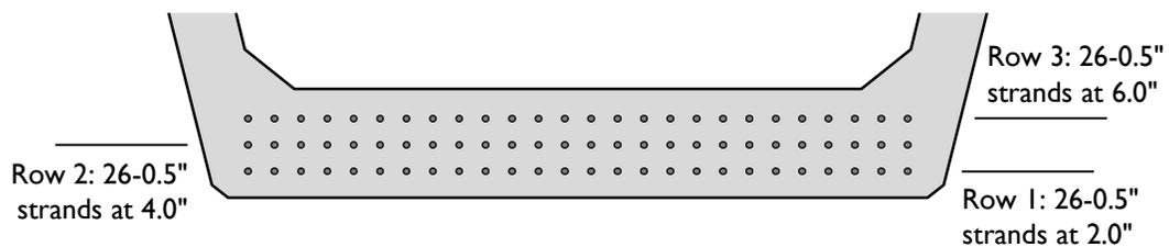
Figure A-7: Prestressing strand positions for Beam 1.
