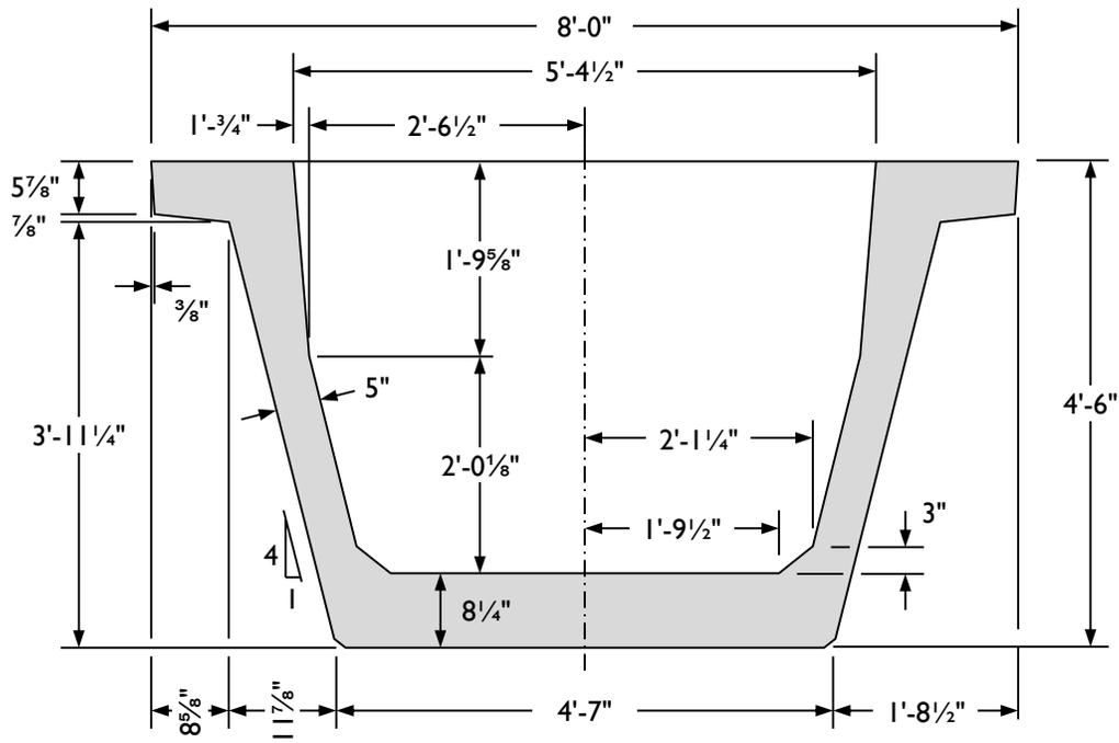
Figure 2-1: Cross-sectional dimensions of the Texas U54 U-Beam.
