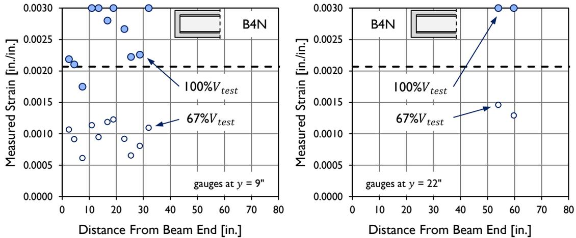
Figure B-42: Strain measured in reinforcing bars during load-testing of specimen B4N.
