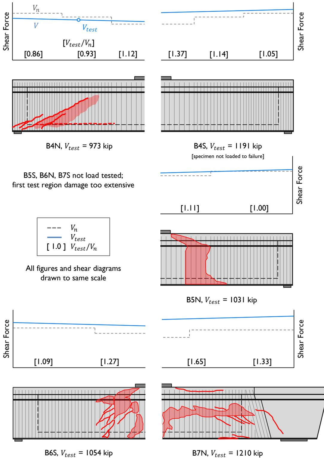
Figure 6-31: Summary of Phase II U-Beam shear tests.
