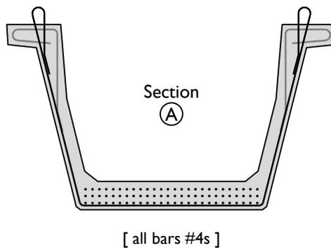
Figure 4-2: (iii) Standard cross section of Beam 1.
