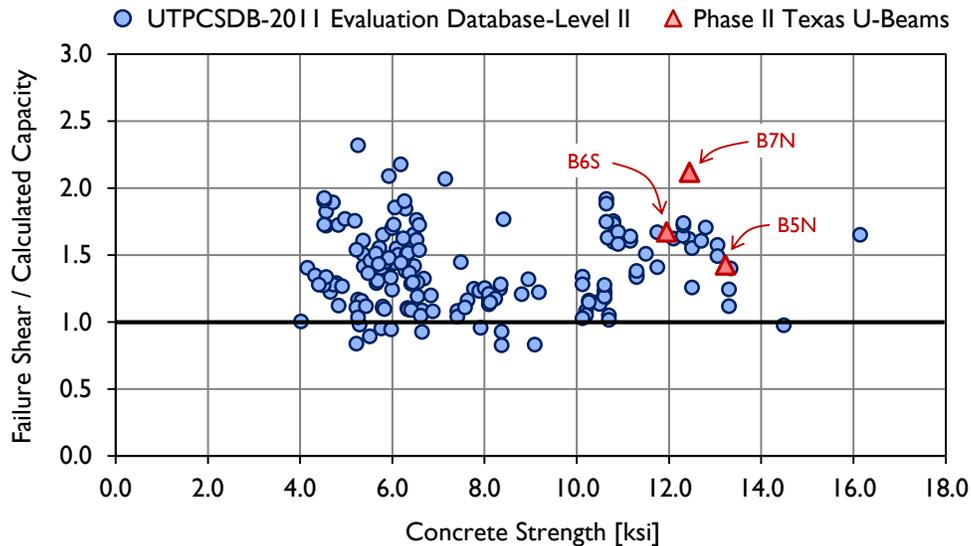
Figure 6-32: Texas U-Beam failure shear-to-calculated shear ratios (capacity calculated using ACI Detailed Method (2008)), compared to other UTPCSDB-2011 data points.
