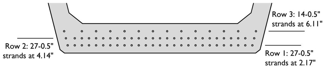
Figure A-4: Prestressing strand positions for Beam 0.
