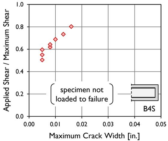
Figure B-30: Maximum crack widths measured in test specimens B4N and B4S.
