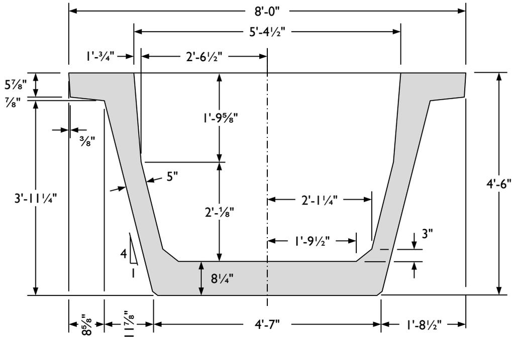
Figure 3-2: Geometry of the Texas U54 beam.
