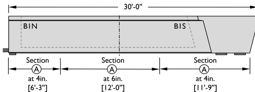
Figure 4-2: (ii) Elevation view of Beam 1.
