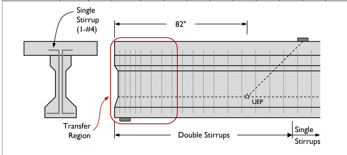
**Table C-17: Reinforcing bar locations in specimens tested by Tawfiq (1995) (2 of 2).**
