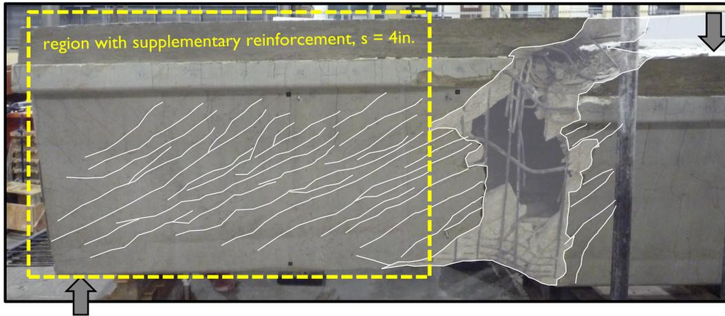
**Figure 5-8: Test region B5N after flexure-shear failure.**
