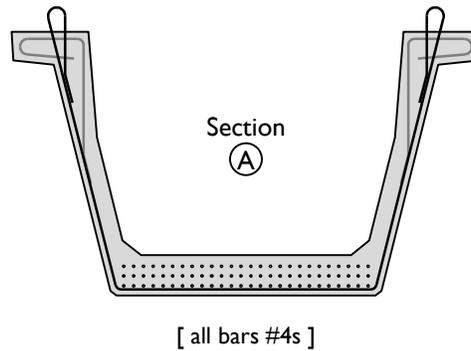
Figure 4-9: (ii) Standard cross section of Beam 3.
