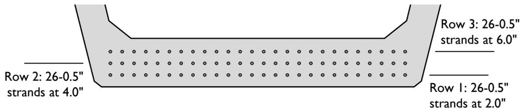
**Figure A-11: Prestressing strand positions for Beam 2.**
