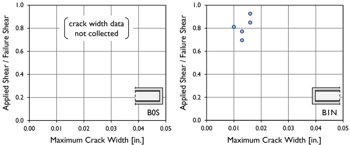
Figure B-27: Maximum crack widths measured in test specimens B0S and B1N.
