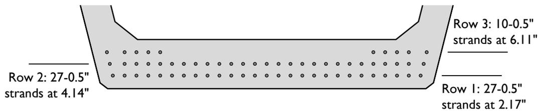
**Figure A-29: Prestressing strand positions for Beam 6.**
