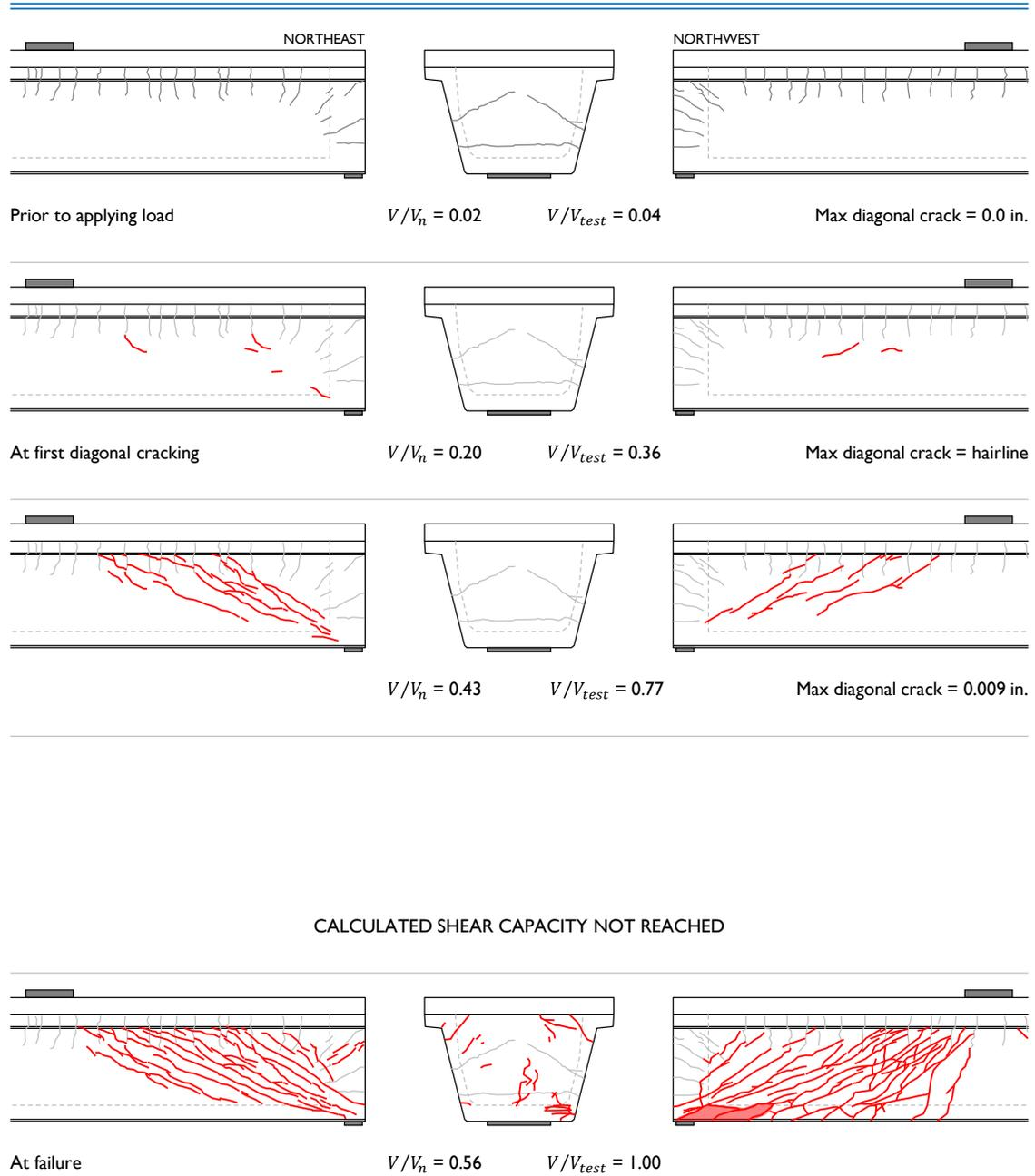
**Figure B-19: Cracks observed during testing of specimen B2N.**
