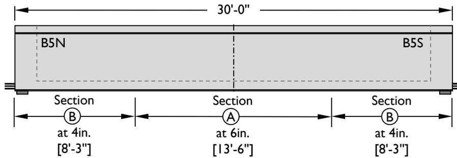
Figure 5-6: (i) Elevation view of Beam 5.
