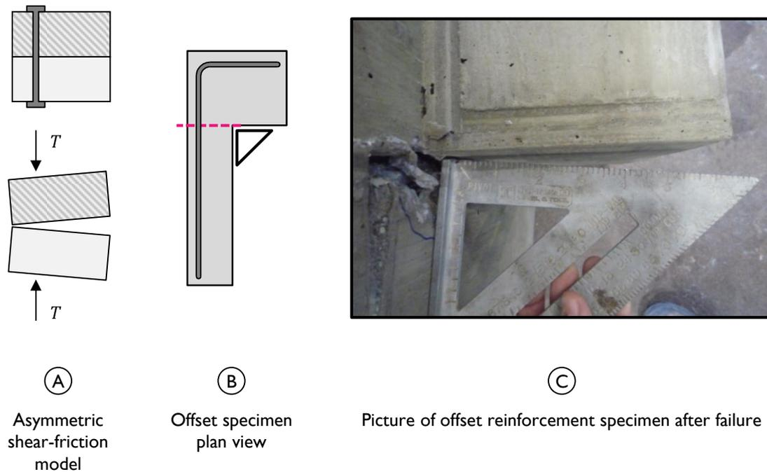
Figure 7-35: Observations of asymmetric opening of shear-friction interface.
