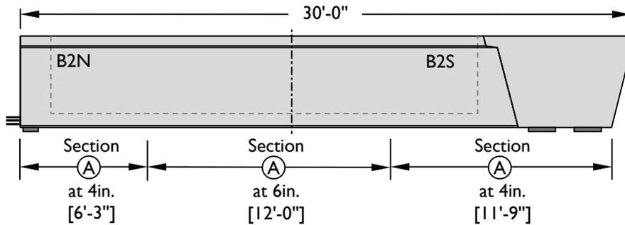
Figure 4-5: (ii) Elevation view of Beam 2.
