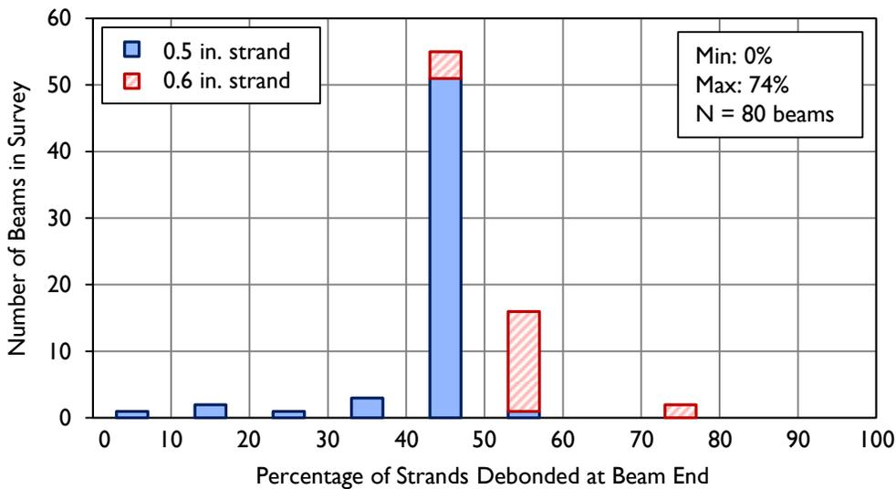
**Figure 3-8: Percentage of debonding in typical Texas U-Beams.**
