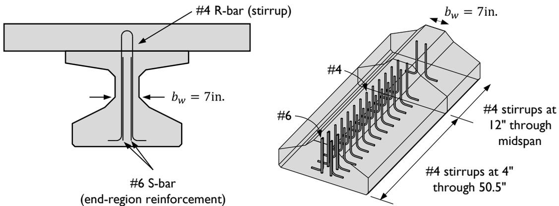
Figure 7-16: Reinforcing bar layout in specimen Tx28-I-D.
