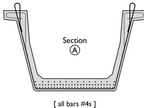
**Figure 4-1: (ii) Standard cross section of Beam 0.**
