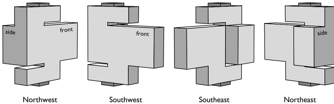
Figure 7-31: Modified push-off specimen viewed from four corners.
