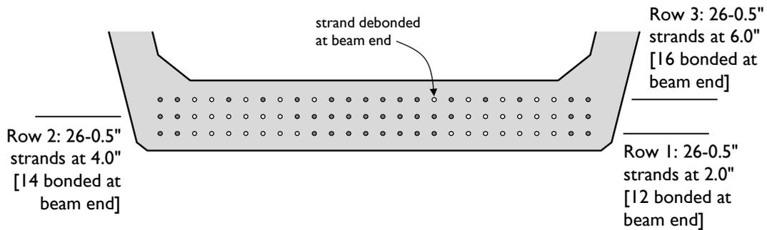
Figure A-15: Prestressing strand positions for Beam 3.
