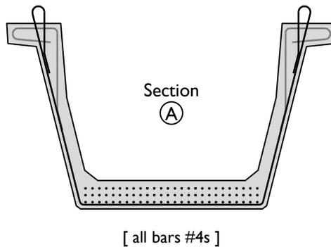
Figure 4-5: (iii) Standard cross section of Beam 2.
