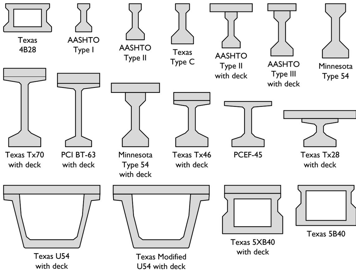
**Figure 7-18: Beam shapes included in the Horizontal Shear Evaluation Database.**
