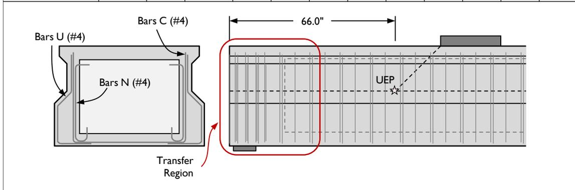
**Table C-6: Reinforcing bar locations in specimens tested by Avendaño (2011) (3 of 3)**
