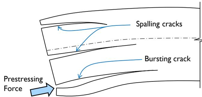
**Figure 2-10: Bursting and spalling deformations (from Dunkman 2009).**
