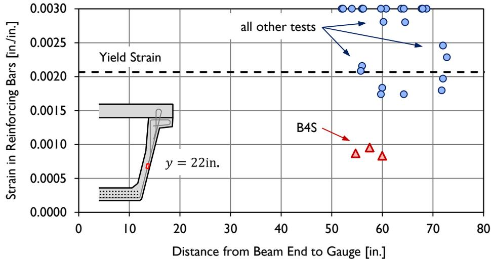
Figure 6-25: Strain in reinforcing bars at maximum load.
