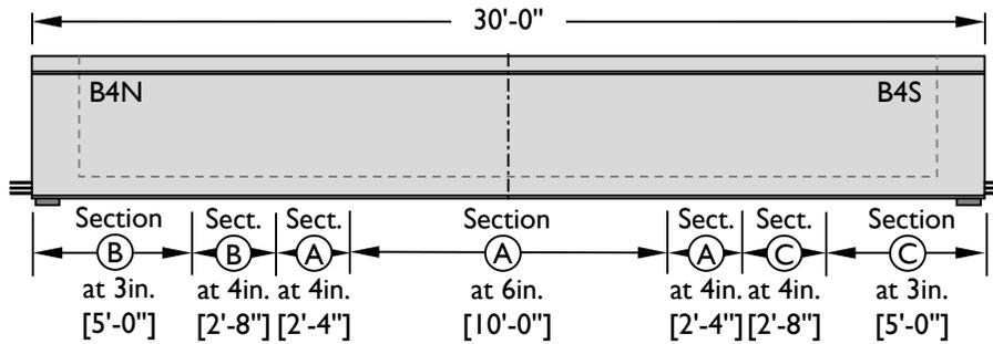
Figure 5-1: (i) Elevation view of Beam 4.
