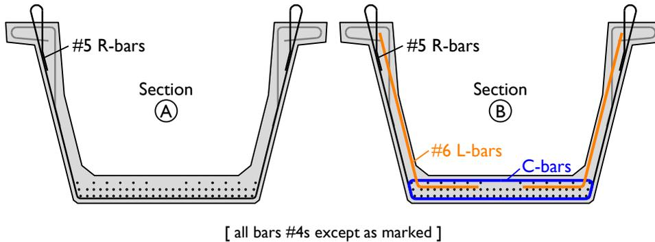
Figure 5-6: (ii) Standard cross sections of Beam 5.
