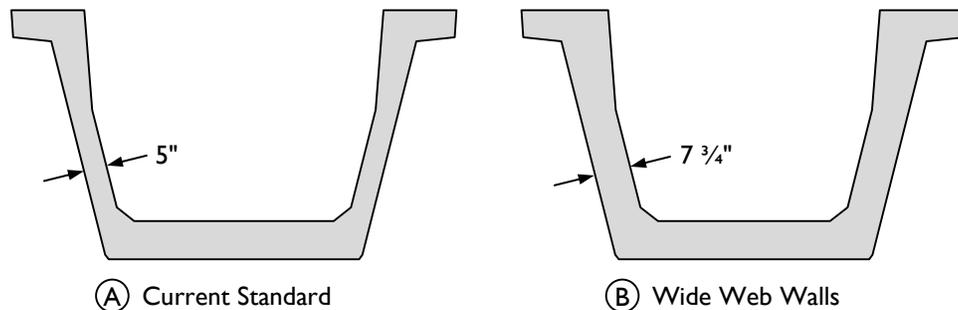
**Figure 3-25: Comparison of (A) standard cross section to (B) cross section with widened web walls.**
