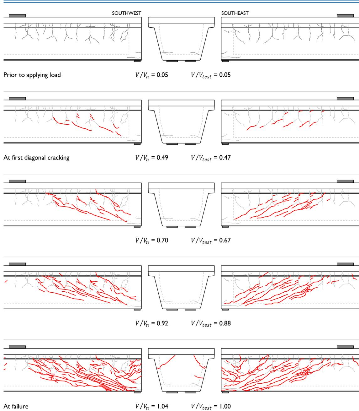
**Figure B-16: Cracks observed during testing of specimen B0S.**
