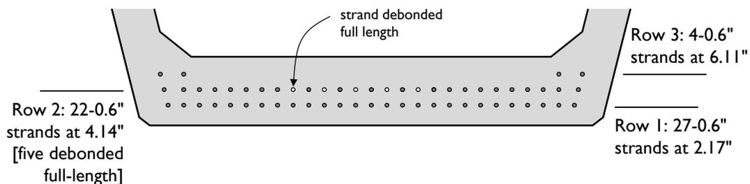
Figure A-33: Prestressing strand positions for Beam 7.
