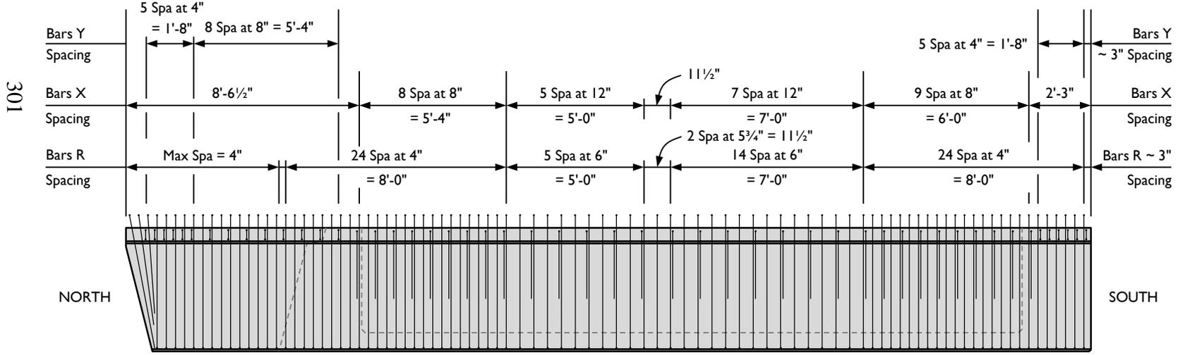
ELEVATION VIEW – Beam 7 Standard Reinforcement
