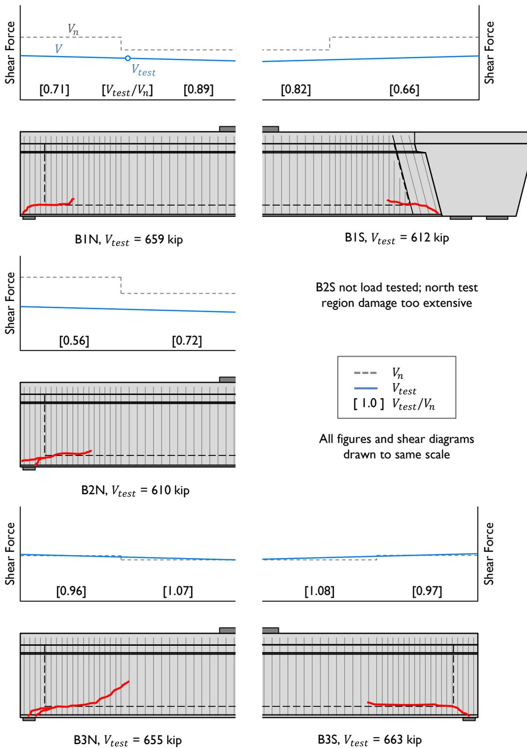
Figure 6-29: Summary of Phase I U-Beam shear tests.
