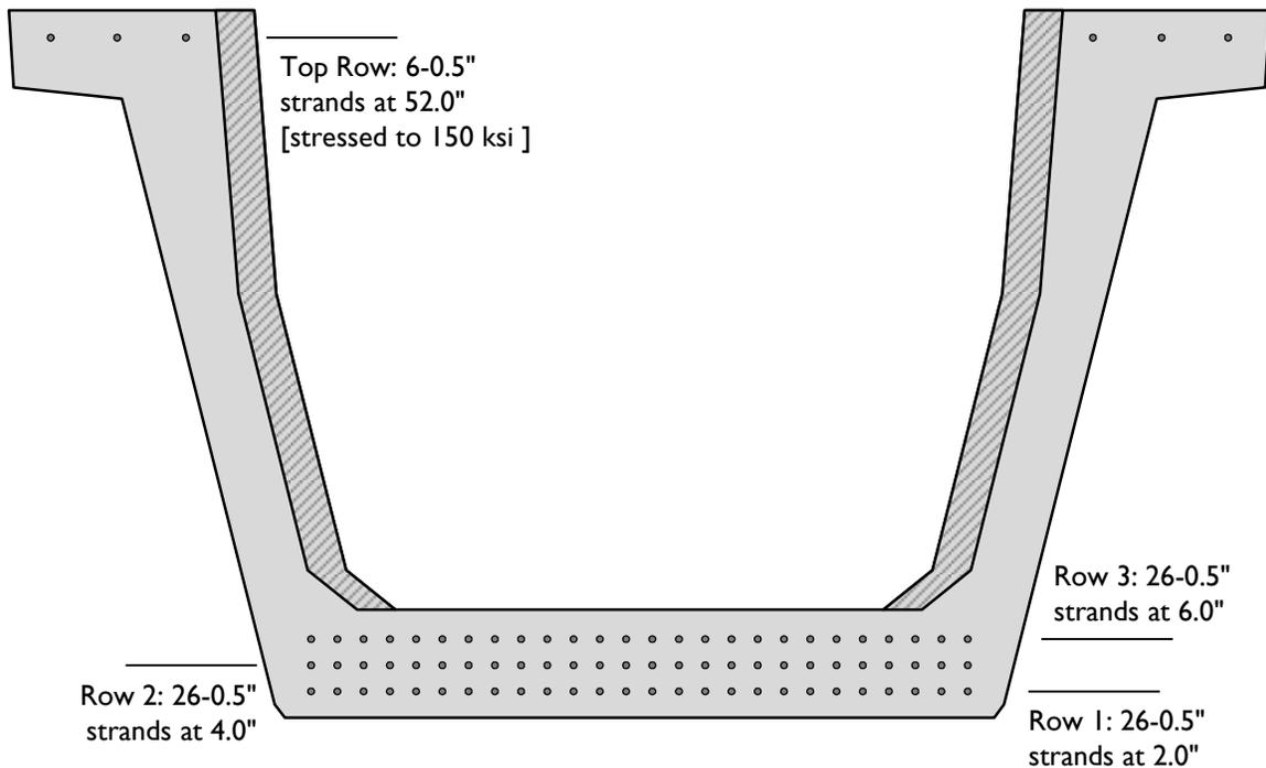
Figure A-19: Prestressing strand positions for Beam 4.
