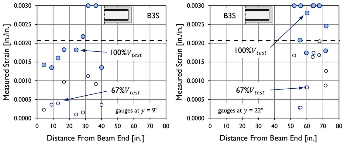
Figure B-41: Strain measured in reinforcing bars during load-testing of specimen B3S.
