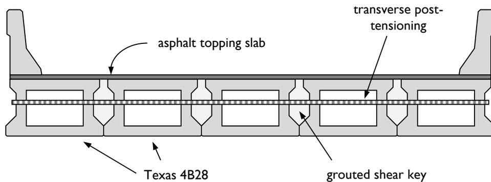
**Figure 2-19: Typical layout of Texas 4B28s in service.**
