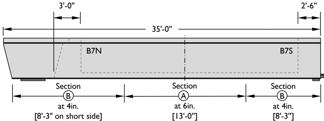
Figure 5-16: (ii) Elevation view of Beam 7.
