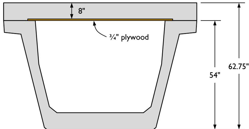
**Figure 3-15: Deck form system used, highlighting  $\frac{3}{4}$ " plywood.**
