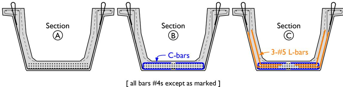
Figure 5-1: (ii) Standard cross sections of Beam 4.
