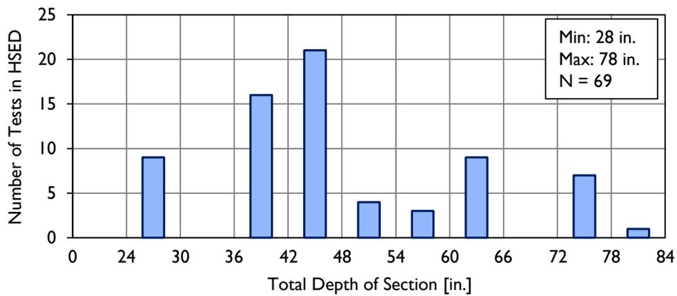
Figure 7-20: Distribution of specimen size in the HSED.
