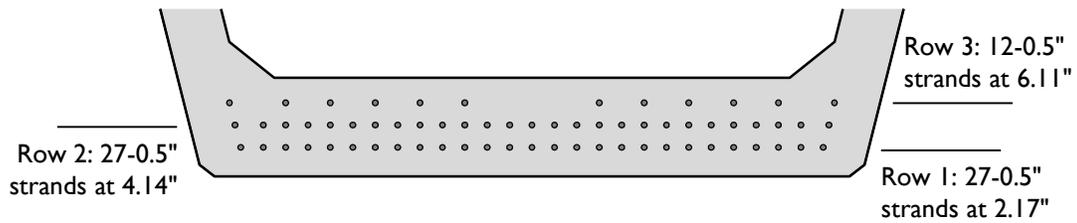
**Figure A-25: Prestressing strand positions for Beam 5.**
