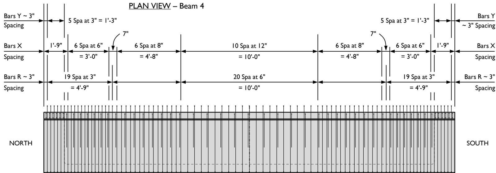
ELEVATION VIEW – Beam 4 Standard Reinforcement
